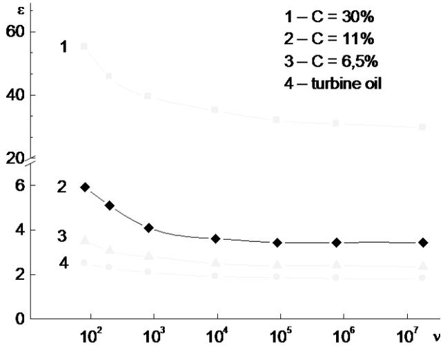
Fig. 1. Frequency dependence of  $\epsilon$  value of MF based on turbine oil.  $T=293$  K.
