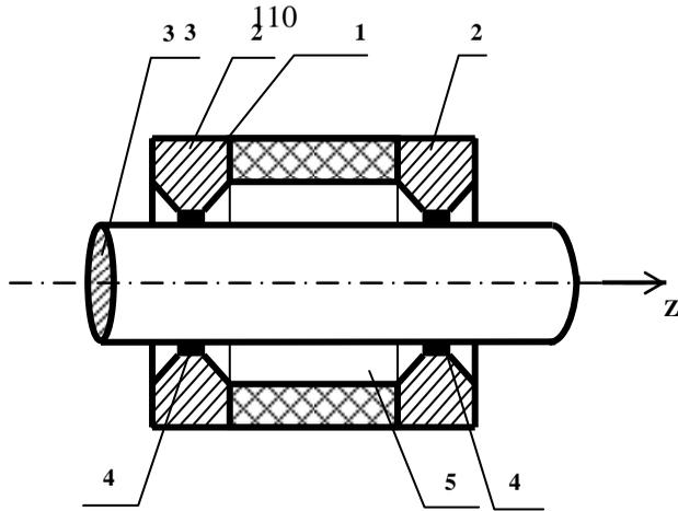
Fig. 2 Magnetic fluids sealant
