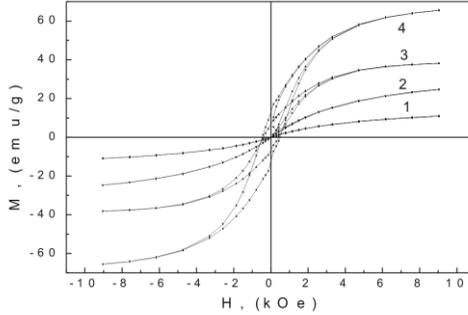
Fig. Room temperature hysteresis loops of carbon fiber matrix with different concentration of cobalt cations in precursor cellulose (mmol/g): 1-2,5; 2-3,1; 3-2,5; 4-3,1 and different final heat-treatment temperature (°C): 1,2-700; 3,4-900
