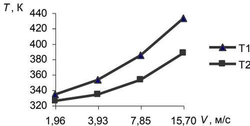
Fig.2 The dependence of the temperature of magnetic fluid on the shaft surface on the linear velocity; T1 – without taking the influence of magnetic field concentrators into account; T2 – taking the influence of magnetic field concentrators into account.
