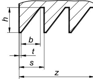
Fig.1 The dimensions of magnetic field concentrators
