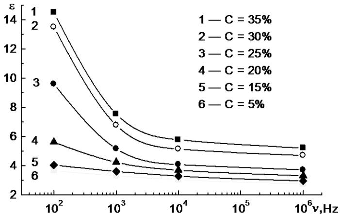
Fig. 4. Frequency dependence of  $\epsilon$  value of MF based on dekanе.  $T=293\text{ K}$ .
