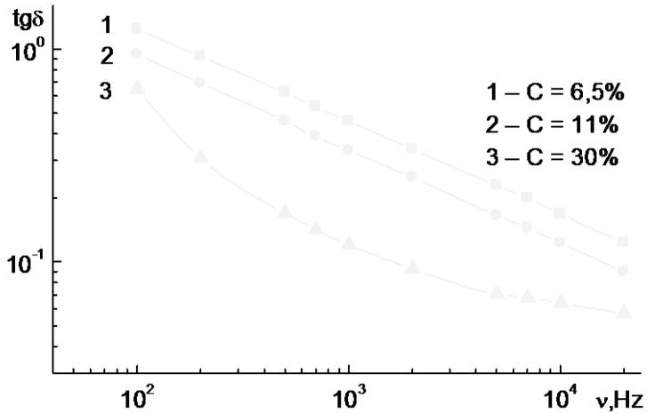
Fig. 3. Frequency dependence of  $\text{tg}\delta$  value of MF based on turbine oil.  $T=293\text{ K}$
