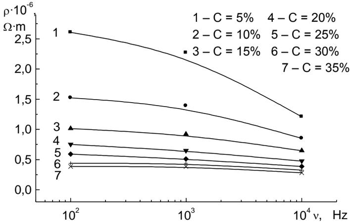
Fig. 5. Frequency dependence of  $\rho$  value of MF based on dekane.  $T=293$  K.
