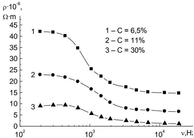
Fig. 2. Frequency dependence of  $\rho$  value of MF based on turbine oil.  $T=293$  K.
