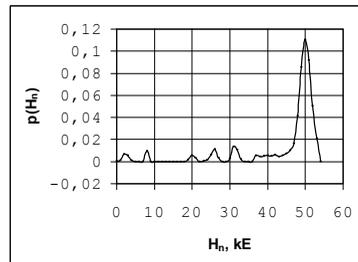
B) Powders from MF on a basis  $\gamma\text{-Fe}_2\text{O}_3$ , from exicator with additional grinding in agate mill.
