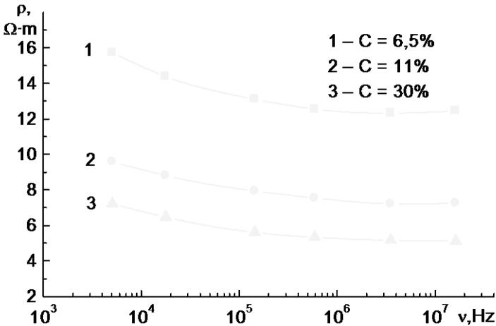
Fig. 6 Frequency dependence of  $\rho$  value of MF based on water.  $T=293$  K.
