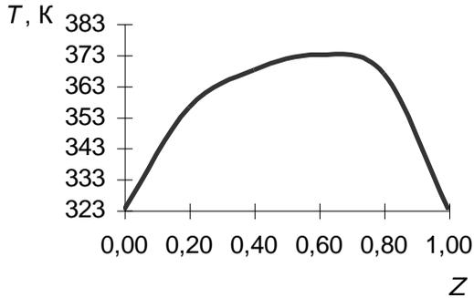
Fig.3 The distribution of temperature between magnetic field concentrators at  $V = 15.7$  m/sec linear speed of shaft.
