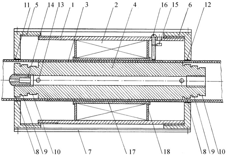
Fig. 1. A cylinder magnetic circuit connected with face covers, 1 – cylinder magnetic circuit, 2 – magnetizing coil, 3 – non-magnetic pipe-line, 4 – water core, 5, 6 – face covers, 7 – tie-rod, 8, 9, 10 – core steps, 11, 12 – through holes surface of face covers, 13 – axis holes, 14 – plug, 15 – plug joint, 16 – retainer screw, 17 – coil sleeve, 18 – check-piece.
